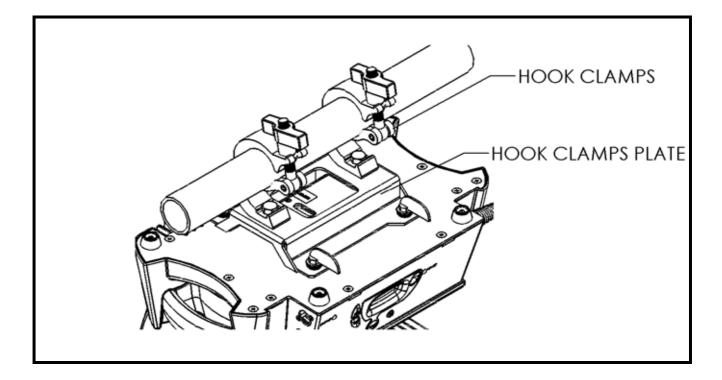
The hook clamps plate is fixed on the top box with 4 flame head fasteners (1/4 turn fasteners).
