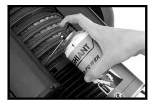
To clean the shutters: Use dry air to clean and a vacuum cleaner to remove dust and other loose particles.
