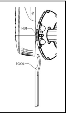
Loose the nuts on both sides, using the special tool. Slide the WARP in the yoke guide (3) until the balancing point is found. Retighten the nuts in the desired position.
