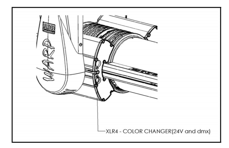
The XLR4-F connector on the motor-house provides DMX data and Power Supply (24Vdc/1A) for an additional device on the WARP. Typical example: a colour changer.
