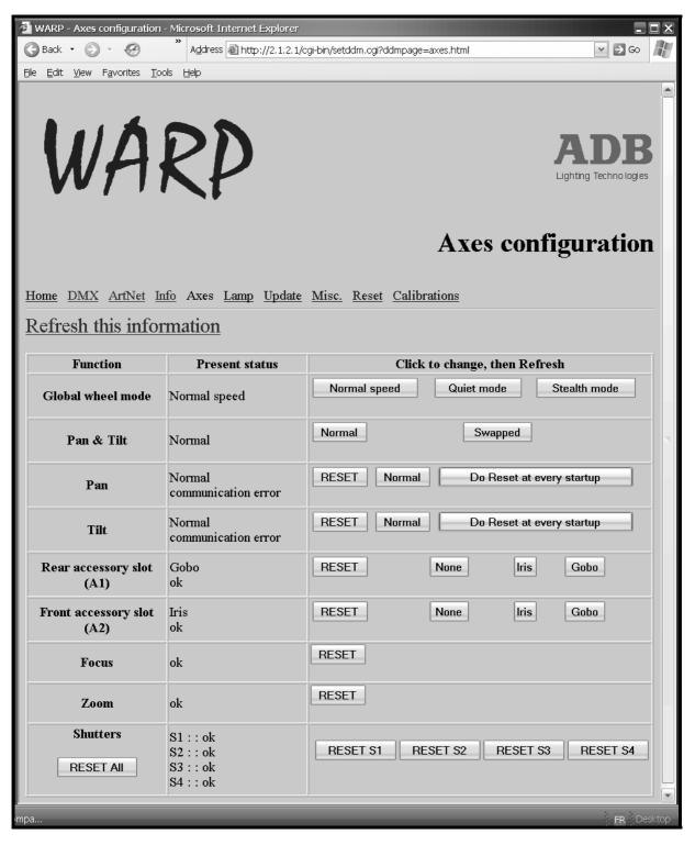
Clicking on one of the functions will immediately send the change to the WARP. Present status will indicate selected parameter and/or the status of the function. Refresh the information before reading the status.
